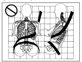
**A:** The shoulder belt is worn under the arm. It should be worn over the shoulder at all times.
